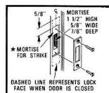
Draw a horizontal line on the jamb where the top of the Lock Front will be when the door is closed Draw a vertical € where center of Lock Front will be. Measure down 5/8" to locate the top of the Strike. Trace an outline of the Strike and mortise the jamb for the Bolt and for the Strike Install Strike.
