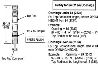
Ready for 84 (2134) Openings Openings Under 84 (2134) For Top Rod cutoff length, deduct OPENING HEIGHT from 84 (2134). Example: Opening = 80 (2032)84 - 80 = 4 or (2134) - (2032) = (102)Top Rod must be cut 4 (102). Openings Over 84 (2134) For Top Rod additional length, deduct 84 (2134)
