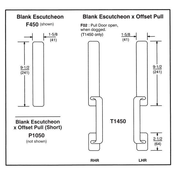
Dimensions given in  $\frac{\text{inches}}{\text{(mm)}}$
