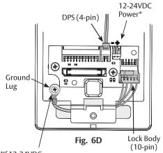
\*If 12-24VDC power harness used, secure its ground (ring terminal) here as well
