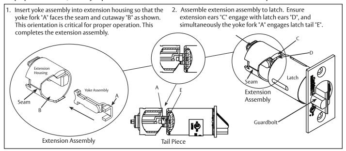
3. After assembly, the seam and cutaway "B" needs to be on the same side as deadlocking guardbolt. Then assemble sleeve to hold both latch and latch extension.
