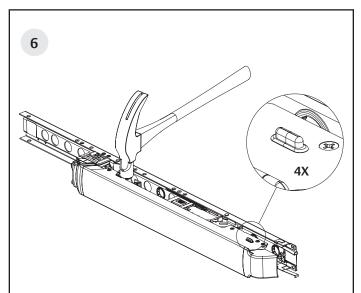
Remove the four wear guides (two on each side) by tapping them with a hammer to pop them out. There will be new wear guides to install in the kit, if these break during removal.
