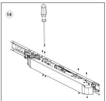
Install push onto push brackets. Secure push onto brackets with four (4) screws on each side.
