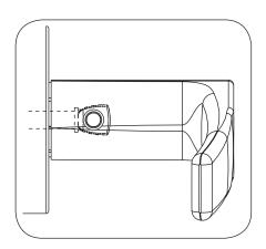
Adjustment bolt fully aligned.
