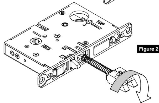
4. Push in latch while holding screwdriver behind latch tail. (Figure 8)
