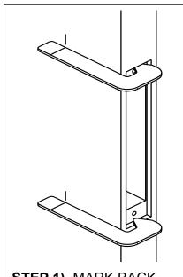
STEP 1) MARK BACK-SET USING GAGE (GAGE GOES INSIDE FRONT POCKET NOT ON DOOR EDGE) (BOTH TOP AND BOTTOM)
