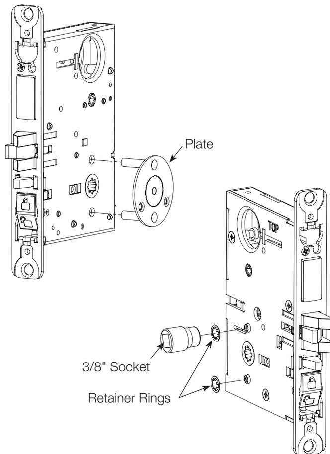
2. Install two (2) retainer rings using 3/8" socket.
