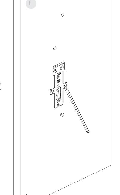
Mark the inner chassis mounting holes.
