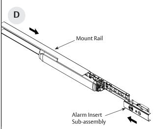
Slide the mount rail until it stops on the dogging slope, then install the alarm insert sub-assembly with the cylinder close to the push. Make sure to press the switch firmly against the trigger mechanism.
