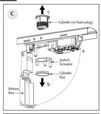
Remove the original cylinder (or foam plug, if ordered without the cylinder):
