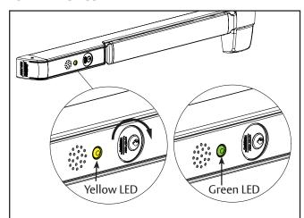
Turn the key clockwise. The LED will flash yellow (PASSAGE) for 15 seconds (default). A quick chirp will sound and the LED will flash green (ARMED) every 30 seconds. Signal indicates unit is armed.
