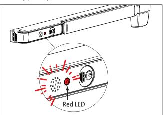
When ARMED, depressing the push rail will activate the alarm. The alarm will sound and the LED will flash red (VIOLATION). The alarm will continue for 2 minutes (default). After 2 minutes, the LED will flash red every 30 seconds until rearmed using the key. Turn the key counter clockwise to deactivate the alarm, then clockwise to rearm.
