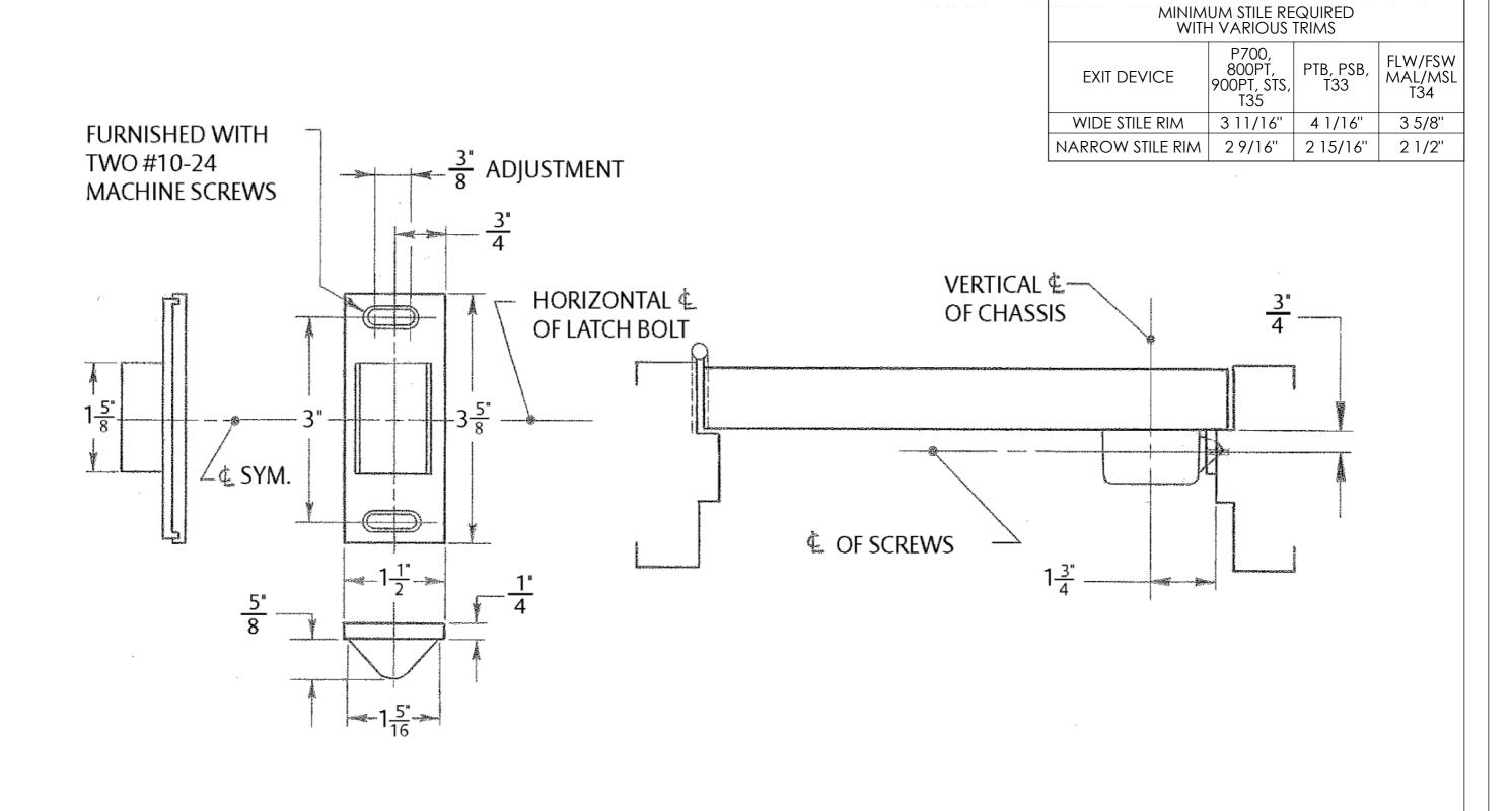
SEE METAL DOOR TEMPLATES TO MOUNT EXIT DEVICE. FRACTIONAL TOLERANCE ±1/64"
