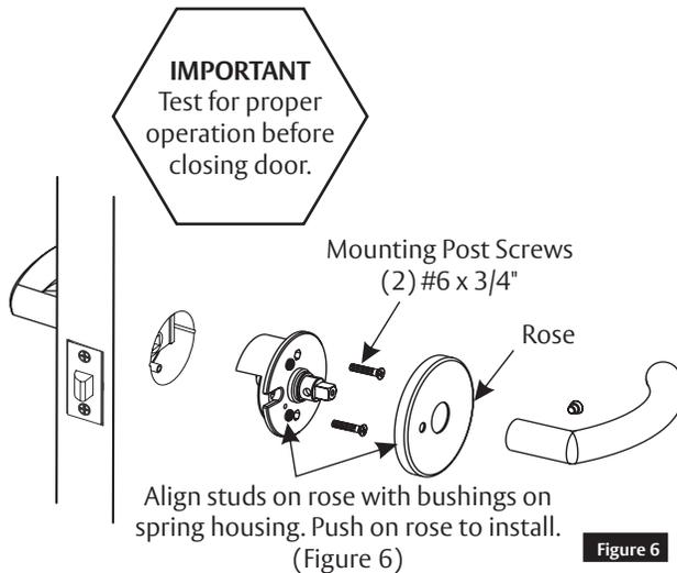
**Note:** Rose to be removed with a flat head screwdriver at notch.
