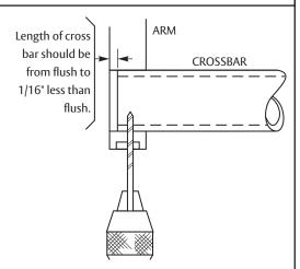
Note: If a shorter crossbar is required, cut crossbar to length and re-drill a 3/16" hole thru one side using hole in arm for locating.
