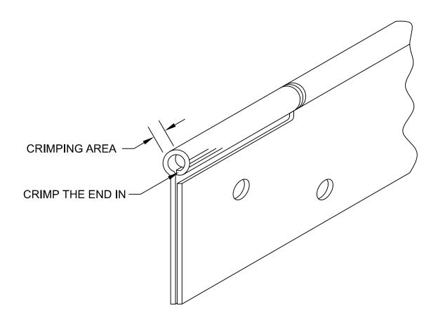
ABH suggests ordering the hinge cut to length at factory. If the hinge is field cut, it will void the warranty.
