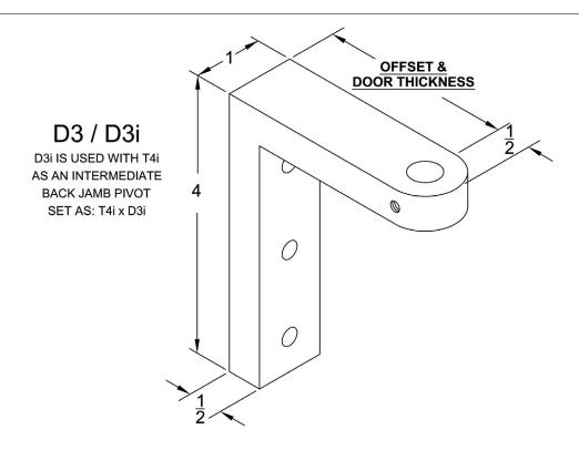
LEFT HAND STANDARD DUTY SHOWN (FOR SET SCREW ACCESS) SCREW: 1-1/4 x #12
