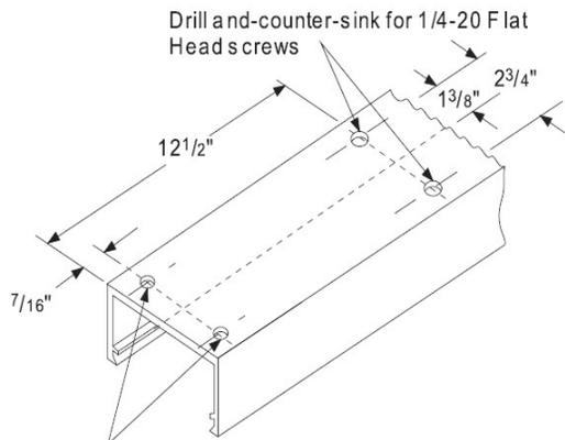
Drill and counter-sink for 10-32 F lat Head screws
