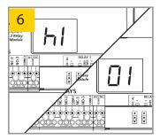
Press<sup>3</sup> INCR to cycle through parameter's values.
