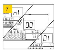
Repeat steps 4-7 until all function parameters are set. Wait 5 seconds for DS1-X to save and display function.
