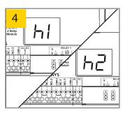
Once desired function is selected, press FUNC to cycle through parameters.
