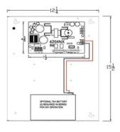
CLASS 2 UL294 RATED ,WITH BATTERY CHARGING CIRCUIT & FIRE ALARM RELAY. THE AUXILLARY CLASS 2 POWER LIMITED OUTPUT SUPPLIES CONTINUOUS DC POWER WHILE A SECOND OUTPUT PROVIDES SWITCHED DC POWER THROUGH THE BUILT IN FIRE ALARM RELAY. FURNISHED IN A 15-1/2" x 12-1/4" x 4-1/2" ELECTRICAL BOX. SEE SERIES 4200 OPTIONS BELOW
