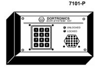
**EDR-101 DELAYED EGRESS CONTROL PANEL** KEYPAD CONSOLE, AUDIBLE ALERT, 3 SECOND NUISANCE / 15 SECOND ALARM DELAY, PROGRAMMABLE CLOCK / DAY SCHEDULER, 3 STATUS OUTPUTS, PROGRAMMABLE ESCORT CODE FOR KEYPAD (OR OPTIONAL KEY SWITCH) INCLUDES 12 VDC 1 AMP POWER SUPPLY, WITH 9 VOLT RECHARGEABLE BATTERY, 3 GANG S/S FLUSH MOUNT PLATE, 3 GANG (IVORY) SURFACE MOUNT BOX, AND 20 FOOT LONG HOOK-UP **CABLES**
