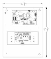
RELAY LOGIC 2-DOOR INTERLOCK CONTROLLERS ARE OFFERED IN STANDARD CONFIGURATIONS WHICH ALLOW FOR ONE DOOR STATUS AND ONE R-E-X INPUT PLUS ONE DPDT LOCK RELAY OUTPUT PER DOOR.
