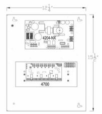
PLC BASED MULTI DOOR, INTERLOCK & MANTRAP CONTROLLERS ARE OFFERED IN STANDARD CONFIGURATIONS WHICH ALLOW FOR ONE DOOR STATUS AND ONE R-E-X INPUT PLUS ONE DPDT LOCK RELAY OUTPUT PER DOOR. A MAXIMUM OF 6-INPUTS AND 4-OUTPUTS CAPABILITY PLUS CUSTOM OPERATIONAL CHARACTERISTICS INCLUDING SEQUENCING AND TIMING MAY BE DESIGNED INTO THE UNIT UPON REQUEST.
