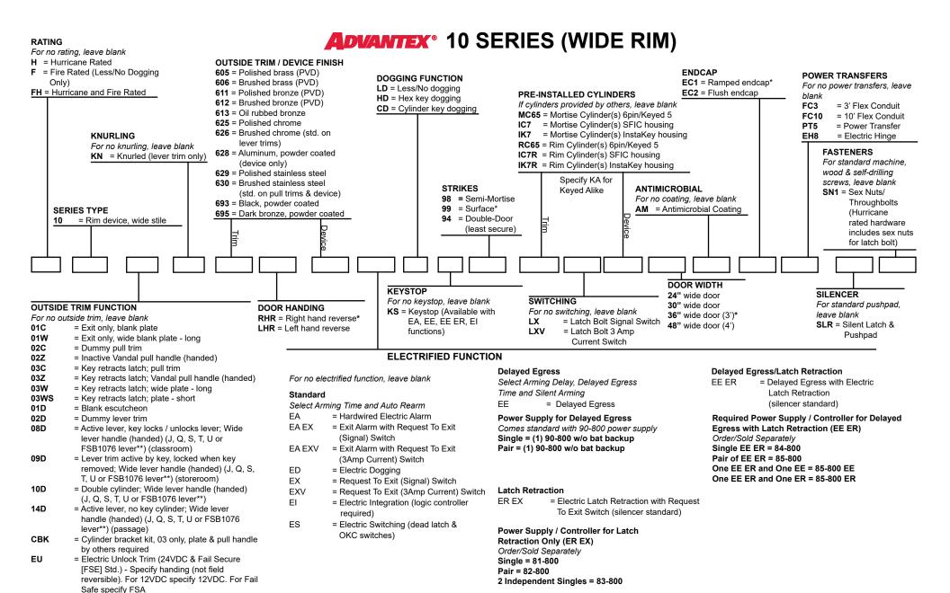
Fire-rated trims must be fail safe (FSA)
