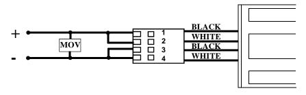
NOTE: TO PROTECT OTHER ELECTRONIC DEVICES IN SYSTEM CONNECT THE SUPPLIED MOV ACROSS THE LEADS AS SHOWN ABOVE.
