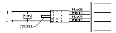
NOTE: TO PROTECT OTHER ELECTRONIC DEVICES IN SYSTEM CONNECT THE SUPPLIED MOV ACROSS THE LEADS AS SHOWN ABOVE.
