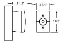
An outlet box should be mounted with reinforcement to withstand load from door
