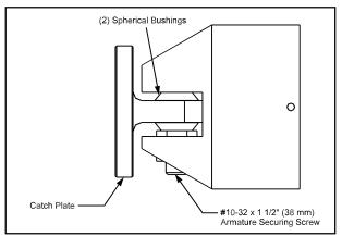
Figure 1. Armature Base Assembly
