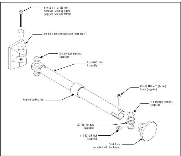
Figure 2. Extension Rod Assembly
