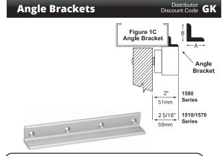
ANGLE BRACKETS: Used as extension on shallow door frames to provide adequate mounting surface. See Figure 1C.
