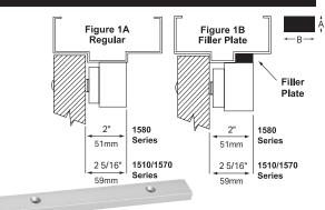
FILLER PLATES: For extension of the stop to provide a proper mounting surface on the underside of the header. See Figure 1B.
