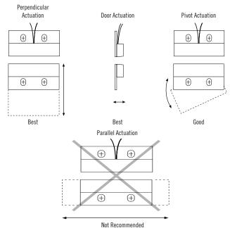
Three configurations are appropriate for interlock applications. The parallel actuation can result in on/off/on signal if the actuator passes by the switch rather than coming to rest in proximity to it. This is NOT a recommended configuration for interlock applications.
