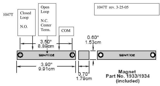
N.C. Normally Closed Contact Terminal Marked Open (Open Loop) N.O. Normally Open Contact Terminal Marked Closed (Closed Loop) COM Common Terminal
