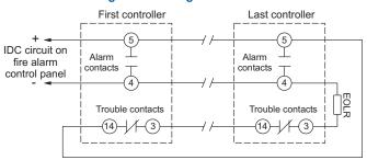
End-of-line resistor required on last device for circuit supervision. Use resistor value specified by the fire alarm panel manufacturer.
