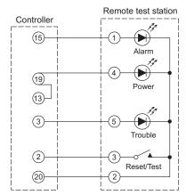
**Note:** For applications where only the Alarm LED and Reset/Test switch is required, wiring the Power LED and Trouble LED is optional.
