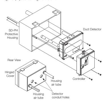
The SD-PH is easy to install and service. The hinged and transparent cover provides ready access to the detector, while keeping its status indicators visible at all times.
