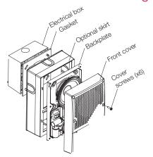
WG4 signals are rated for outdoor use and are suitable for indoor or outdoor applications on walls or ceilings. For surface-mounting in outdoor or wet applications, appliances must be mounted to an Kidde 74347U electrical box. In dry conditions, they are compatible with standard 4-inch by 1½-inch deep electrical boxes. When using the optional
