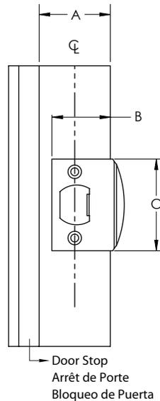
Dimension B & C should be used as reference only. Due to tolerances actual door jamb prep dimensions will vary. Using the strike plate outline edges and locate screw holes on strike with center line on jamb.
