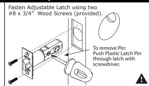
The Adjustable Latch is factory shipped with a 2¾" backset position. Remove pin and slide spindle hub forward for a 2¾" backset, then reinsert the pin in the hole at the back of the latch as shown.
