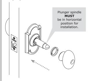
**Step 2.** Tighten knob set screw after placing knob on stem.
