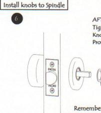
AFTER INSTALLATION: Tighten Set Screws on Knob with Allen Wrench Provided.
