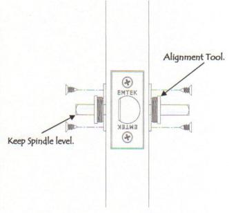
Remember to Remove Plastic Alignment Tool after Flanges are installed.
