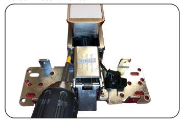
**6.** PUSH THE TWO TABS ON THE LBM BRAKET INTO THE EXISTING HOLES IN THE EXIT DEVICE HEAD.
