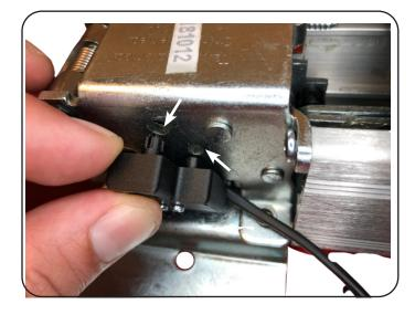
8 INSTALL (1) 60754 CAP ON TO LATCHBOLT ROLL PIN.
