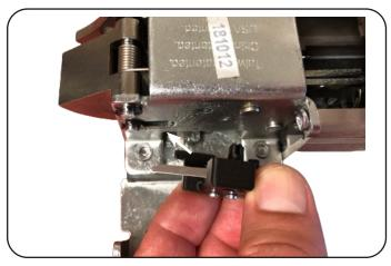
7. CONFIRM SWITCH ARM IS UNDERNEATH RIM LATCH PIN. INSTALL (1) 40266 SCREW INTO TOP HOLE ON LBM BRACKET TO SECURE BRACKET TO EXIT DEVICE HEAD.
