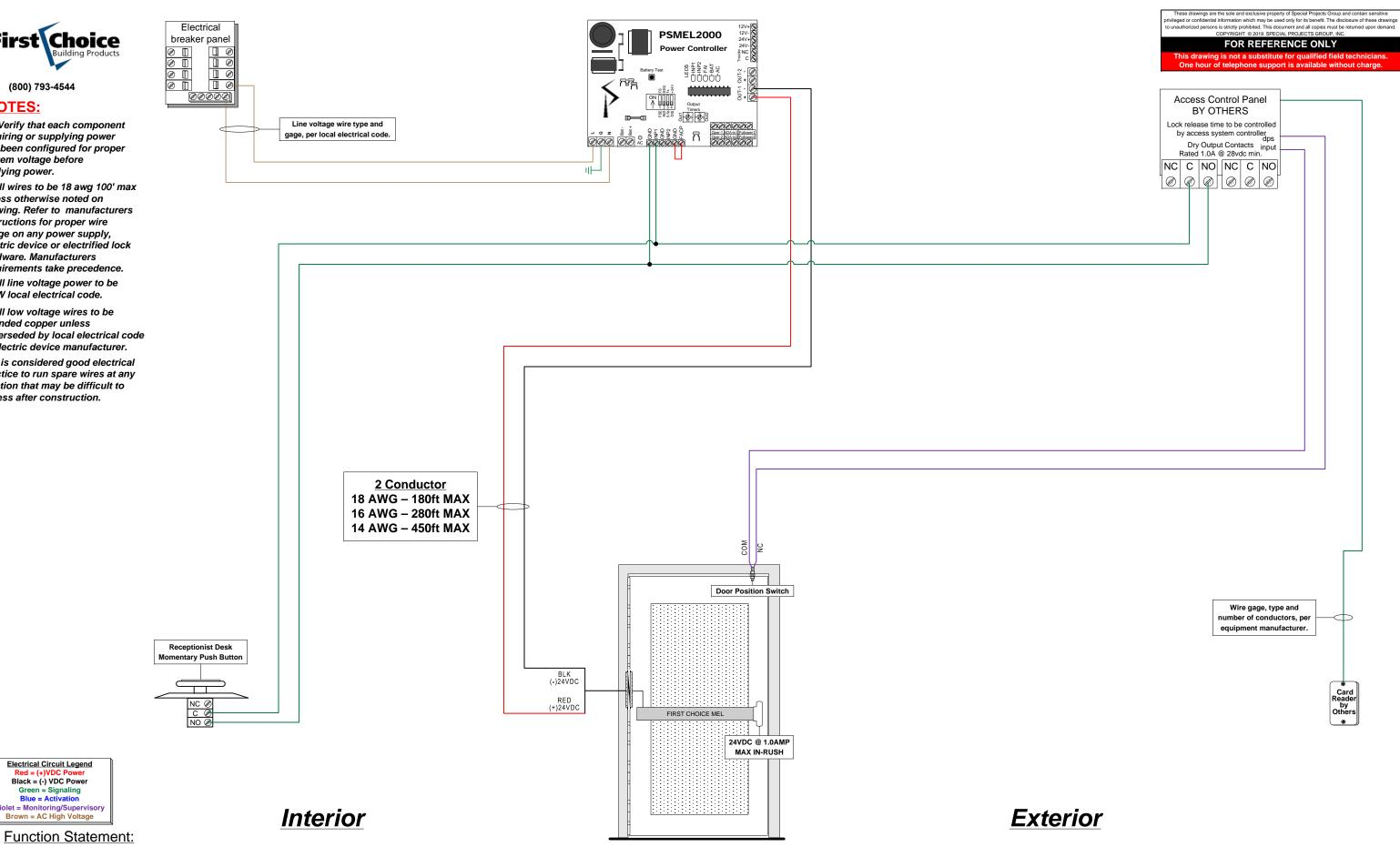
From exterior - locked condition: Access by presenting valid credential at reader interface to retract electric exit device latchbolts. Receptionist push button to unlock door for visitor entry. From exterior - unlocked condition: Door to remain locked unless electric exit device held retracted by access control system or receptionist desk push button control. From interior - locked condition: Free egress at all times by means of exit device.
