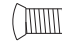
COVERS MOUNTING SCREW (#8-32 X 5/16" WITH #6 PH. OV. U' CUT HD. MACH. SCREW, 14 PCS)
