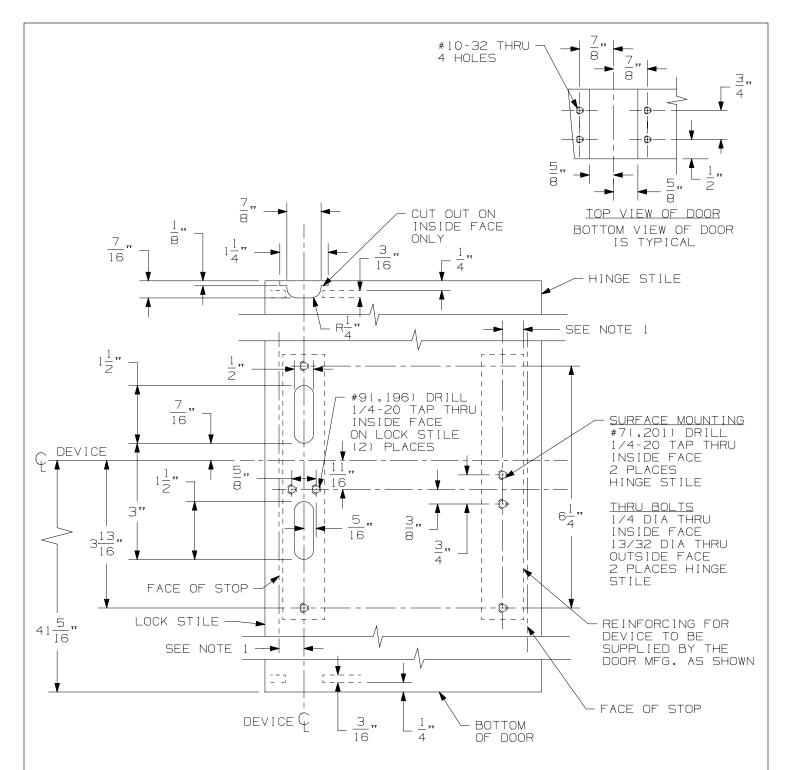
NOTES: 1. THE DIMENSION FROM THE FACE OF THE STOP TO CENTERLINE OF HOUSING IS 3/4" MIN. FOR MEDIUM AND WIDE STILE DOORS, HOUSING MAY BE CENTERED ON STILE. THE CENTERLINE OF THE LATCHES CAN HAVE THE SAME CENTERLINE OR IT CAN VARY TO SUIT DOOR CONDITIONS.
