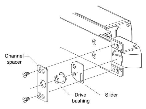
For EO devices, remove channel spacer
