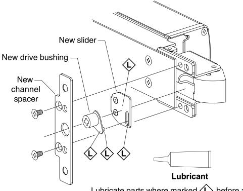
Lubricate parts where marked (L) before assembly
