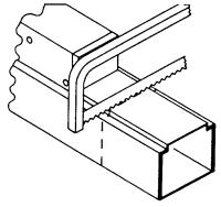
NOTE: FACTORY RECOMMENDS SAWING RATHER THAN GRIND CUT TO SIZE. GRINDING CAN DAMAGE THE FINISH OF THE DEVICE AND SAWING RESULTS IN LESS DAMAGE TO THE **DEVICE'S FINISH.**
