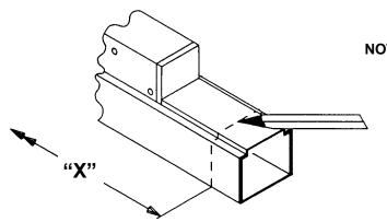
**NOTE: BE SURE CHANNEL COVER IS PUSHED SNUG TO TOUCHBAR PRIOR TO MARKING OR CUTTING TO SIZE**
