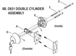
Double Cylinder: Screw ¼" bolts (F) thru housing (E), into housing (D) engaging tailpieces (L) with the vertical slot in the dead bolt.
