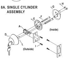
Single Cylinder: Screw ¼" bolts (F) thru plate \*(E) into housing (D) and tighten. Engage tailpiece (L) with thumbtum (G). Fasten thumbtum (G) to plate (E) with short machine screws (H). \*NOTE: Align plate with the large holes below the small holes a shown. For a 1½" diameter bored hole, the 3 dimples should face into the door. For a 2½" diameter bored hole, the circular ridge should face into the door.
