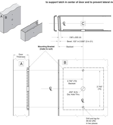
For metal doors installations, suitable reinforcement is required to support latch in center of door and to prevent lateral movement
