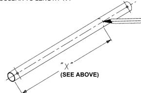
B) CUT CROSSBAR TO MARKED DIMENSION AND REMOVE BURRS.
