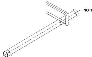
NOTE: FACTORY RECOMMENDS SAWING RATHER THAN GRIND CUT TO SIZE. GRINDING CAN DAMAGE THE FINISH OF THE DEVICE AND SAWING RESULTS IN LESS DAMAGE TO THE DEVICES'S FINISH.
