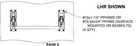
6) ATTACH ROD GUIDE BRACKETS TO DOOR ON VERTICAL & EQUIDISTANT BETWEEN THE LATCHES AND DEVICE HEAD.
