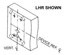
4) IF USING OUTSIDE TRIM, PREPARE DOOR USING SEPARATE TRIM DIRECTION SHEET. FOR SEXBOLT INSTALLATIONS, DRILL 3/8" DIAMETER HOLES ON TRIM SIDE OF DOOR ONLY (SEE DIAGRAM BELOW).
