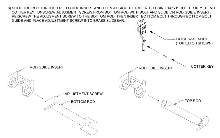
9) TURN ADJUSTMENT SCREW UNTIL IT IS APPROXIMATELY 1/2" INTO THE VERTICAL ROD. SWING RODS SO THAT THE ADJUSMENT SCREW IS IN THE BRASS SLIDEBAR IN THE ACTIVE HEAD AS SHOWN BELOW.
