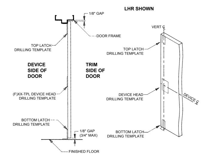
3) PREPARE HOLES FOR DEVICE, STRIKE AND LATCHES. FOR DEVICES WITH TRIM FUNCTIONS, PREPARE THE HOLE(S) ON THE DEVICE TEMPLATE DESCRIBED IN THE CHART BELOW. AFTER DRILLING HOLES, REMOVE THE DRILLING TEMPLATE.
