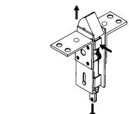
C. PUSH UP ON ROD CONNECTOR. THE LATCH BOLT WILL RETRACT AND REMAIN RETRACTED.
