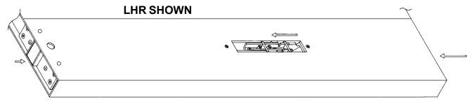
8) CHECK THE PROJECTION OF THE BOTTOM BOLT. WITH THE TOP LATCH BOLT RETRACTED THE BOTTOM BOLT SHOULD NOT BE PROJECTING FROM THE BOTTOM OF THE DOOR, BUT SHOULD STILL BE HELD BY THE BOTTOM BOLT GUIDE. IF THE BOLT IS PROJECTING FROM THE DOOR, TURN THE BOTTOM ADJUSMENT SCREW CLOCKWISE; IF IT IS INSIDE THE DOOR, LINE UP THE BOTTOM BOLT WITH THE BOLT GUIDE AND TURN THE BOTTOM ADJUSTMENT SCREW COUNTER-CLOCKWISE.
