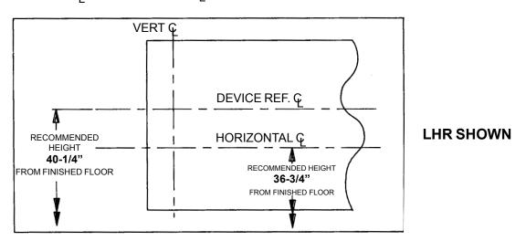
3) MARK LOCATION OF RELEASE BRACKET ACCESS HOLE ON VERTICAL & AT TOP OF DOOR AS SHOWN BELOW.
