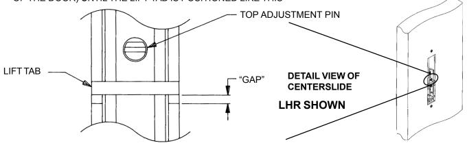
6) TURN THE TOP ADJUSMENT PIN COUNTER-CLOCKWISE UNTIL THE LIFT TAB MOVES TOWARDS THE BOTTOM OF THE DOOR AND CLOSES THE "GAP".
