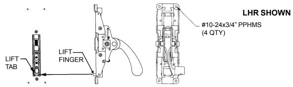
3) REMOVE CROSSBAR RETAINER SCREW AND ROUNDED WASHER FROM XX CROSSBAR ARMS. SLIDE THE CROSSBAR OVER BOTH THE ACTIVE AND INACTIVE ARMS AND ATTACH WITH CROSSBAR RETAINER
