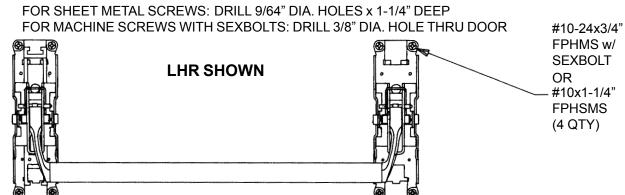
5) INSTALL TOP STRIKE USING TWO #10-24x3/4" FPHMS, REFER TO DRILLING TEMPLATE DT-1301.
