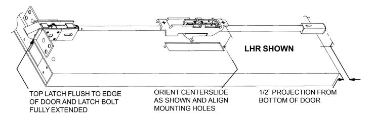
4) PICK UP THE ENTIRE ASSEMBLY AND INSERT BOTTOM ROD AND BOLT ASSEMBLY INTO TOP LATCH CUT-OUT. SLIDE ASSEMBLY THRU DOOR UNTIL THE TOP LATCH SEATS INTO THE MATING PREPARATION. ATTACH CENTERSLIDE, TOP LATCH, AND BOTTOM BOLT GUIDE TO DOOR USING SCREWS LISTED BELOW: TOP LATCH: #10-24x3/4" FPHMS (6 QTY)
