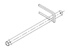
NOTE: FACTORY RECOMMENDS SAWING RATHER THAN CUT GRIND TO SIZE. GRINDING CAN DAMAGE THE FINISH OF THE DEVICE AND SAWING RESULTS IN LESS DAMAGE TO THE DEVICE'S FINISH.
