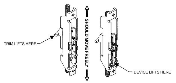
B. USING A SMALL FLAT-BLADE SCREW DRIVER, PUSH IN GENTLY ON THE TWO ADJUSTMENT PINS AND TURN. THE ROD CONNECTOR SCREW WILL ROTATE. (THIS IS THE VERTICAL ROD ADJUSTMENT FEATURE).
