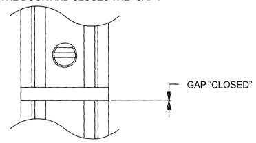
7) LIFT UP ON THE LIFT TAB UNTIL THE TOP LATCH BOLT IS FULLY RETRACTED. THEN, ATTEMPT TO SLIDE THE CENTERSLIDE THE OPPOSITE DIRECTION, THE CENTERSLIDE SHOULD NOT MOVE AND THE TOP LATCH BOLT SHOULD REMAIN IN THE RETRACTED POSITION. IF NOT, TURN THE TOP ADJUSMENT PIN ONE QUARTER TURN COUNTER-CLOCKWISE AND TRY AGAIN. REPEAT UNTIL THE TOP LATCH BOLT REMAINS RETRACTED.
