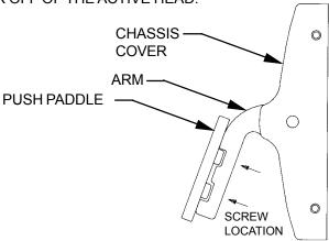
2. AFTER INSTALLING THE ACTIVE HEAD AND MAKING ANY REQUIRED ADJUSTMENTS. SLIDE THE ARM THROUGH THE CUT-OUT IN THE CHASSIS COVER AND INSERT THE AXLE AS SHOWN BELOW. THEN REASSEMBLE CHASSIS COVER TO ACTIVE HEAD WITH THE FOUR SCREWS REMOVED ABOVE.
