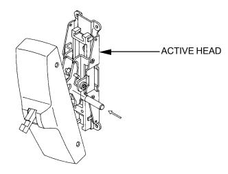
3. AFTER ASSEMBLING THE CHASSIS COVER TO THE ACTIVE HEAD, RE-INSTALL THE PUSH PADDLE TO THE ARM USING THE SOCKET FLAT HEAD SCREWS AND THE 1/8" HEX WRENCH, MAKING SURE THAT THE PUSH PADDLE DOES NOT WOBBLE OR IS NOT TWISTED ON THE ARM.
