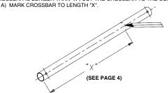
B) CUT CROSSBAR TO MARKED DIMENSION AND REMOVE BURRS.
