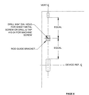
FOR DEVICES ON DOORS OVER 8'0" TALL, TWO ROD GUIDE BRACKETS SHOULD BE PLACED EQUALLY BETWEEN THE TOP LATCH AND DEVICE HEAD.
