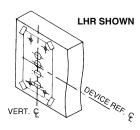
4) IF USING OUTSIDE TRIM, PREPARE DOOR USING SEPARATE TRIM DIRECTION SHEET. FOR SEXBOLT INSTALLATIONS, DRILL 3/8" DIAMETER HOLES ON TRIM SIDE OF DOOR ONLY (SEE DIAGRAM BELOW).
