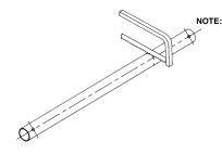
NOTE: FACTORY RECOMMENDS SAWING RATHER THAN GRIND CUT TO SIZE. GRINDING CAN DAMAGE THE FINISH OF THE DEVICE AND SAWING RESULTS IN LESS DAMAGE TO THE DEVICES'S FINISH.
