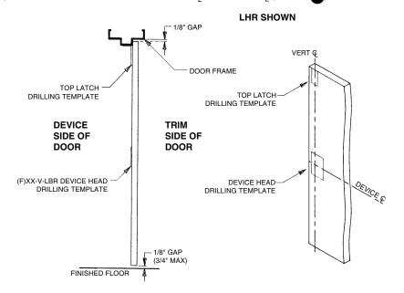
PAGE 12 PAGE 3 3) PREPARE HOLES FOR DEVICE, STRIKE AND LATCHES. FOR DEVICES WITH TRIM FUNCTIONS, PREPARE THE HOLE(S) ON THE DEVICE TEMPLATE DESCRIBED IN THE CHART BELOW. AFTER DRILLING HOLES, REMOVE THE DRILLING TEMPLATE.
