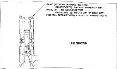
3) REMOVE CROSSBAR RETAINER SCREW AND ROUNDED WASHER FROM XX CROSSBAR ARMS. SLIDE THE CROSSBAR OVER BOTH THE ACTIVE AND INACTIVE ARMS AND ATTACH WITH CROSSBAR RETAINER SCREW AND ROUNDED WASHER.
