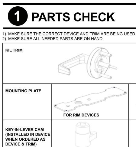
**MOUNTING SCREWS** (#10-24x3/4" FPHMS - 2 QTY) 0 FOR RIM DEVICES FOR VERTICAL DEVICES FOR RIM DEVICES FOR VERTICAL DEVICES (SHIPPED WITH RETAINING RING)
