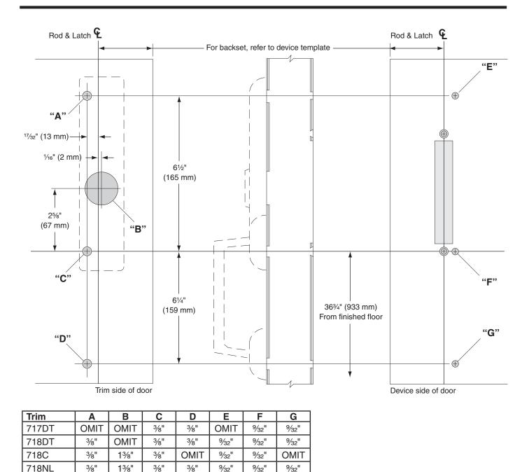
• For height from finished floor, refer to device template.
