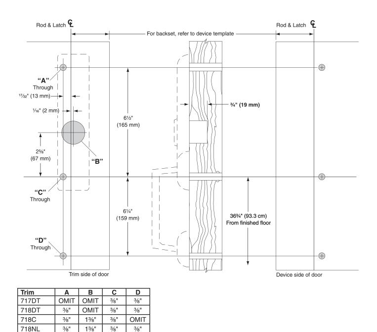
• For height from finished floor, refer to device template.
