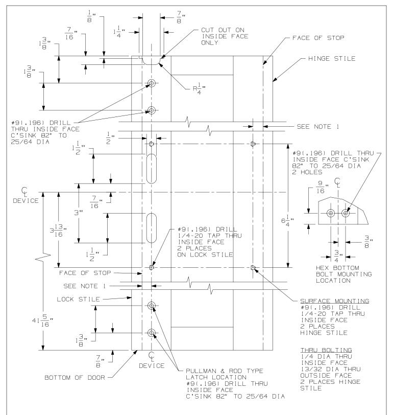
NOTES: 1. THE DIMENSION FROM THE FACE OF THE STOP TO CENTERLINE OF HOUSING IS 3/4" MIN. FOR MEDIUM AND WIDE STILE, HOUSING MAY BE CENTERED ON STILE. THE CENTERLINE OF THE LATCHES CAN HAVE THE SAME CENTERLINE OR IT CAN VARY TO SUIT DOOR CONDITIONS.
