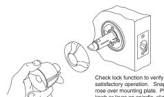
satisfactory operation. Snap rose over mounting plate. Place knob or lever on spindle, slide to locking button, depress button and push knob or lever until button engages hole.
