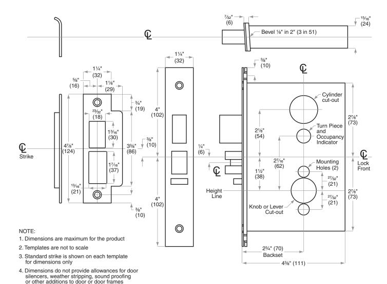
M-Series locks meet all requirements for installations in doors and frames prepared in accordance with ANSI specifications A156.13, 1994 ANSI Standards:
